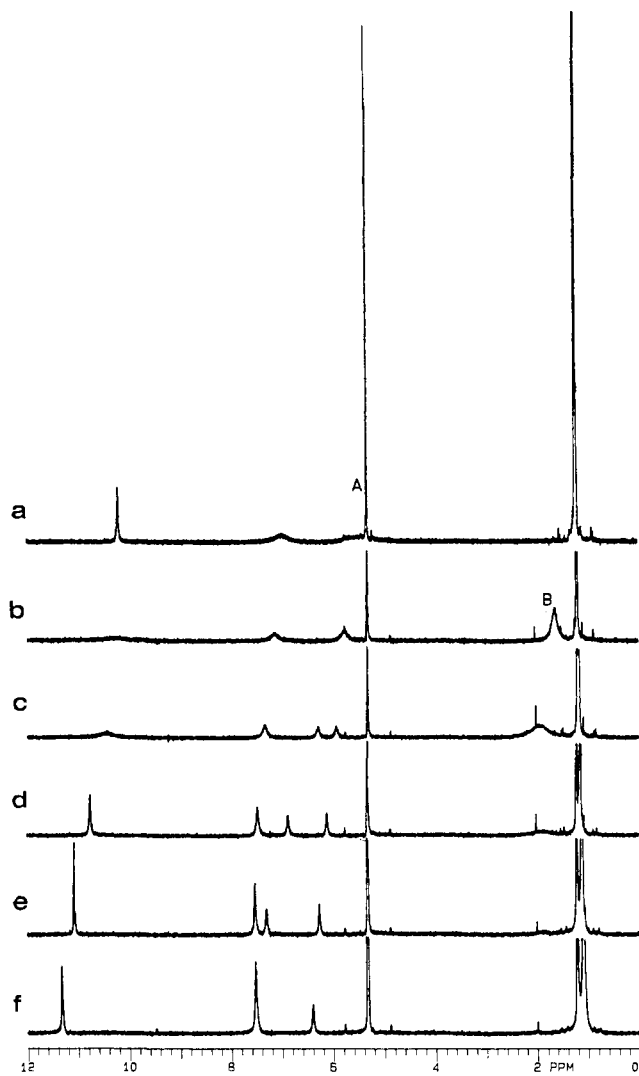
Figure 2. ^1\text{H} NMR spectra as a function of temperature for compound 7c in \text{CD}_2\text{Cl}_2 : (a) spectrum in dry solvent at 20^\circ\text{C} and (b–f) spectra in undried solvent at 0 , -20 , -40 , -60 and -80^\circ\text{C} , respectively. A and B mark the resonances of \text{CHDCl}_2 and water, respectively.
